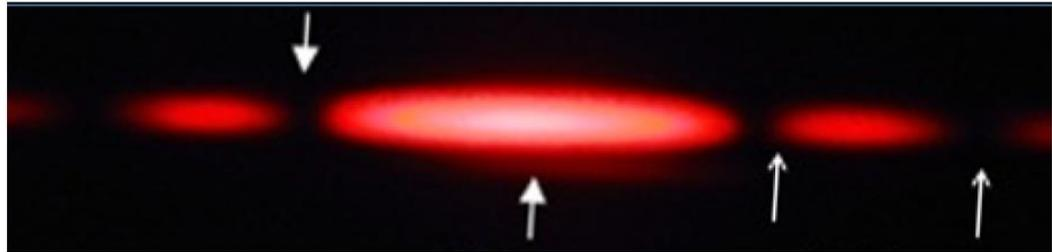
8. In **Double slit**, the resulting interference pattern for the double-slit will also include a diffraction pattern due to the individual slit. The intensity of the total pattern is simply the product of the two functions:
